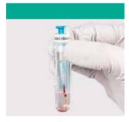
Within 2 minutes insert Sample Collector into the cuvette and close the cuvette with the reagent cap. Do not press down the turquoise inner part of the reagent cap. Run the test within 2 hours.
