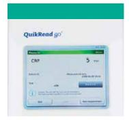
The result appears on the display when the measurement is completed and the cuvette automatically rises from the measurement well.
